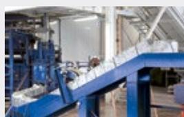
**Balers:** for compacting light-weight FE metals into standard-sized bales for steelworks; cuts freight costs & speeds up the charging process at steelworks
