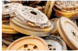
**Foundry scrap:** incl. light/medium scrap, machine castings, nodular cast iron, trimming & cupola scrap
