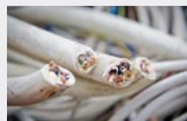
**Cutting mills:** the cable sheaths are removed from the copper wire & the copper recovered
