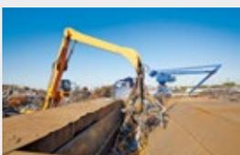
**Shears:** machines (up to 1,400t cutting force) and excavators with hydraulic shears; for cutting up particularly large and heavy materials (e.g. railway tracks or rail wagons)
