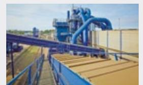
**Shredder:** ten shredders, including two large 6,000-horsepower shredders; recovery of raw materials according to type using diverse automated and manual stages
